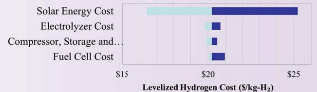
Cost sensitivity for hydrogen produced in the solar PV powered fueling station
