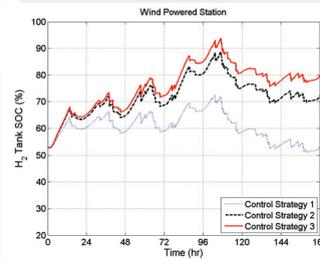
State of charge of the hydrogen storage tank for one week operation, station powered by wind
