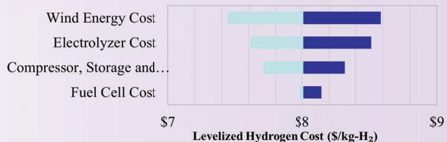
Cost sensitivity for hydrogen produced in the wind powered fueling station
