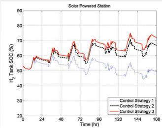
State of charge of the hydrogen storage tank for one week operation, station powered by PV
