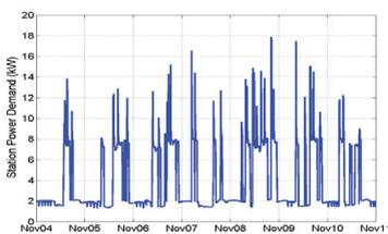
UCI hydrogen station electric load over a week
