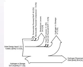
Sankey diagrams of energy fluxes for wind and solar PV powered stations using control strategy 3.
