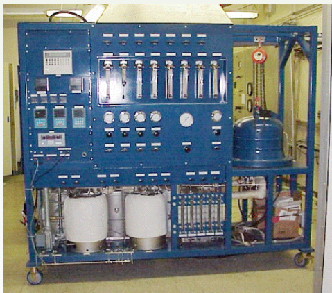
Fig. 1 Front view of the test stand. Its dimension is approximately 8 feet wide, 4 feet deep, and 7 feet tall.
