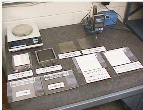
Fig. 2 The necessary components to assembly a single cell. Anode, cathode electrode, matrix, and electrolyte are shown as tapes before loading onto the end plates.
